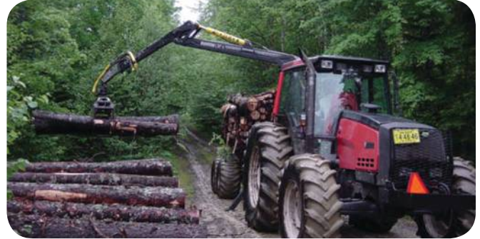
Valmet tractor and log trailer used to forward wood from selection and shelterwood harvesting operations
