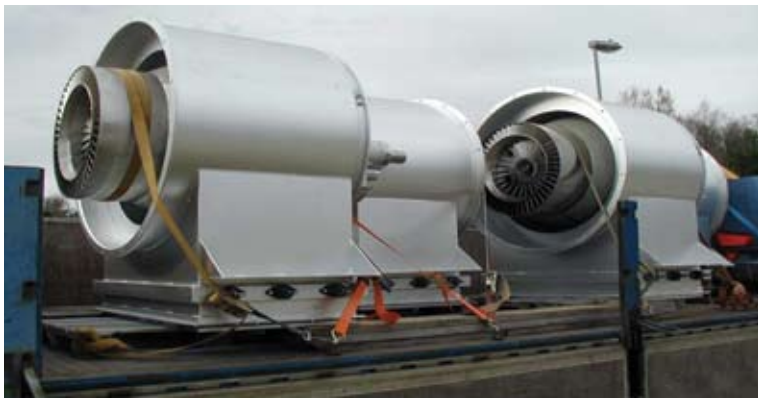
Four of Tall Oil's 25 Mega Watt burners, manufactured by Varnetesnisk Service, one of Sweden's foremost wood-powder burner manufacturers.
