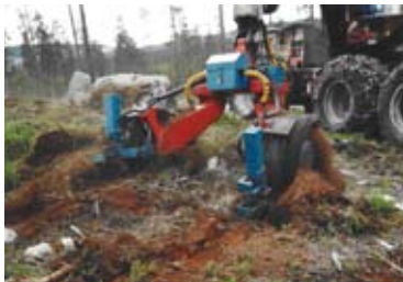
Figure 4 - Seeding system mounted on a processor frame
