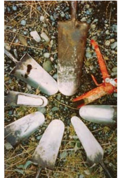
The unique design of a flattened thick tapering blade, straight shank and bullet-rounded edge was the birth of the Treeplanter spade. This tool is unquestionably the most successful planting tool ever introduced, and thousands of units are still sold annually. The early runs at Spear & Jackson were specified to be hard-edged to 47-48 on the Rockwell C scale and lasted longer than later tools.
