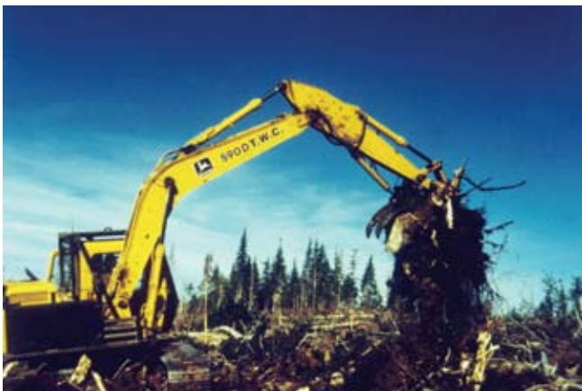
Figure 6. Stumping with an excavator.
