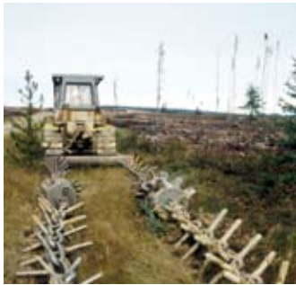
Figure 5. Crawler tractor pulling chains
