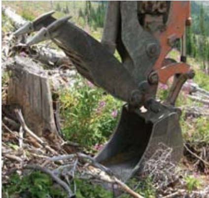
Figure 1. Toothed bucket with a hydraulic thumb used for mounding
